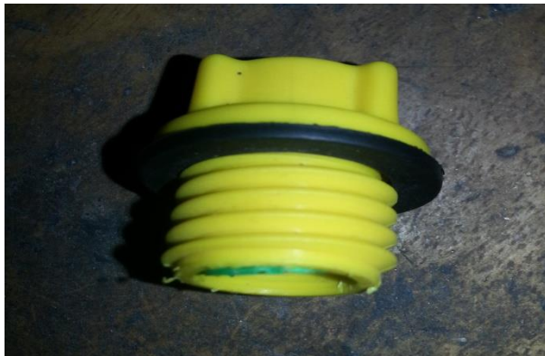
Fig.4: Vent cap of battery
